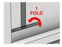
Insert the folded lift strap into the bottom bar spline. The shade might have to be lifted by hand slightly to fit the spline in.
