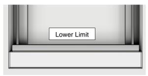
If the strap wanders to much or does not look aligned while the shade was moving, <u>finely</u> adjust the strap left or right and repeat the movement to the upper and lower limit until the strap is properly aligned and the movement looks good.
