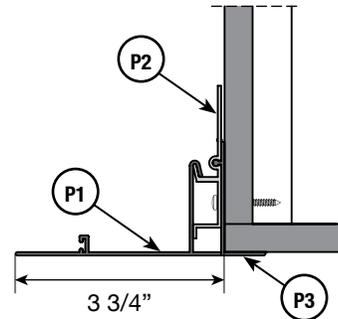
When bottom enclosure is cut down a brush strip will be inserted by Sun Glow to protect the fabric from the cut edge.
