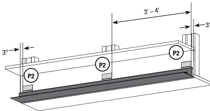
Hangers (P2) are provided as a standard. Each hanger should be placed 3" from either end of the pocket. Additional hangers should be placed every 3' - 4' evenly spaced along the pocket wall.
