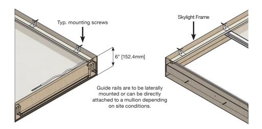
At least 6" [152.4mm] of mounting depth is required to properly install the Nimbus Shade System.
