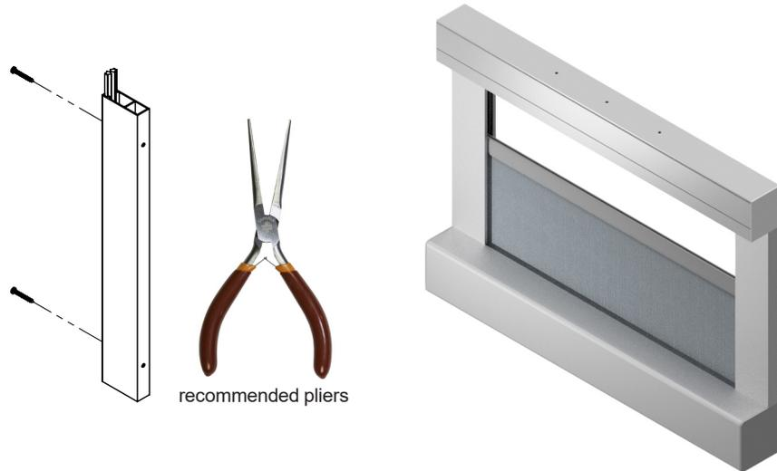
Cables should be positioned inside the channels and free of obstructions, after mounting the side channels, prior to adding tension to the system.
