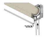
(3) Insert the flat guard into the mounting bracket on the idle end until you here an audible click.
