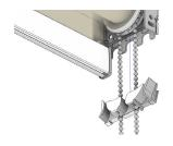
(2) Then insert the chain guard into the mounting bracket until you here an audible click.
