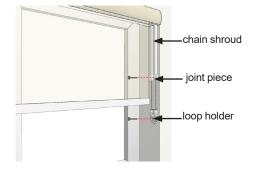
The loop holder and joint piece must be affixed to a wall or window frame.
