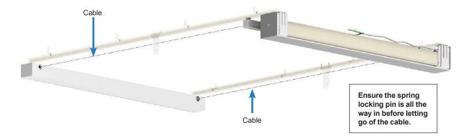
On the end of each cable there is a metal cable connector that is intended to be attached to the square bottom bar. Slide each of the cable connectors into the square bottom bar channel on either side. A plier can be used to help pull the connector through the channel if needed.
