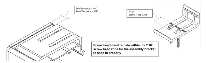
Insert the front edge of the V-102 Assembly Bracket onto the front lip of each V-102 Mounting Bracket, as shown in the diagram below. Starting from one side, push / twist the bracket until the back edge of the V-102 Assembly Bracket snaps into the bottom tab of the V-102 Mounting Bracket. Repeat this process for next bracket.
