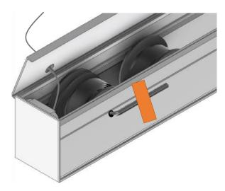
Carefully lift the spring box into the other side of the skylight window frame. The spring box should be installed in a position where the cables are in line and parallel with the fabric.
