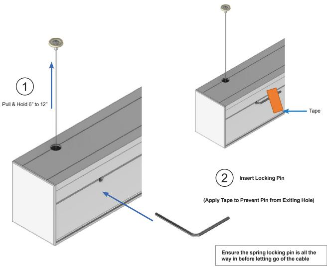
The spring locking pin is meant to take the load of the constant force provided by the springs. Apply the same locking method to the other side of the spring box.
