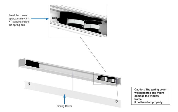
Once finished snap the spring cover back onto the spring box leaving the cables hanging from the spring box.
