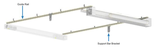
Slide each of the bottom bar guides on either end of the square bottom bar. Starting on one side wall mount the guide rail (L-rail Mounts) inside of the skylight frame. Repeat the process for the other guide rail.
