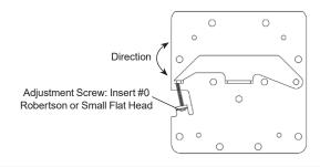
To adjust shade level if window is not square, follow the steps below. Turn the small Adjustment Screw on the Adjustable End Bracket either clockwise to raise the shade or counter clockwise to lower the shade until the shade is level.
