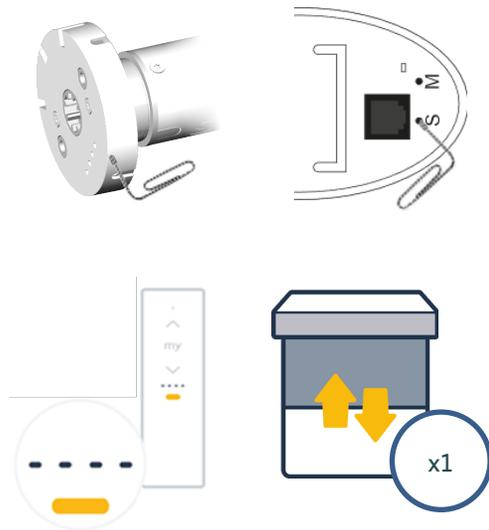
*Radio reception of the motor is reduced in Programming Mode, keep remote(s) within 5 feet of the motor head while programming.*
